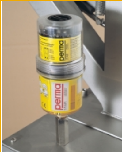
Detail of the auto-lubrication system.
